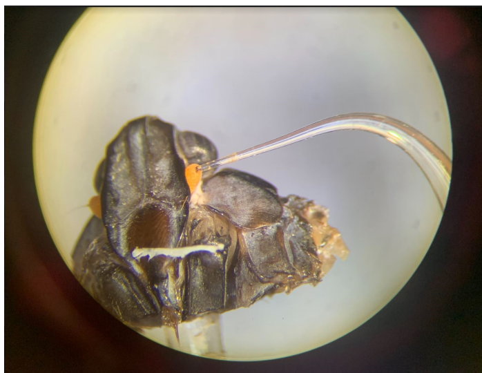
Figure 1. A glass saline electrode connecting to an SLF antenna.
