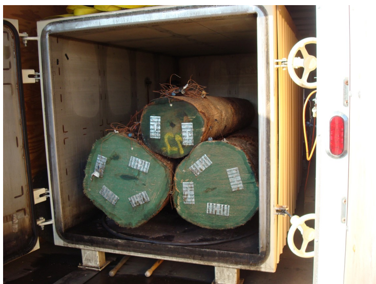
Figure 1. Vacuum steam treatment includes initial processing of white oak logs grouped in a steel chamber
