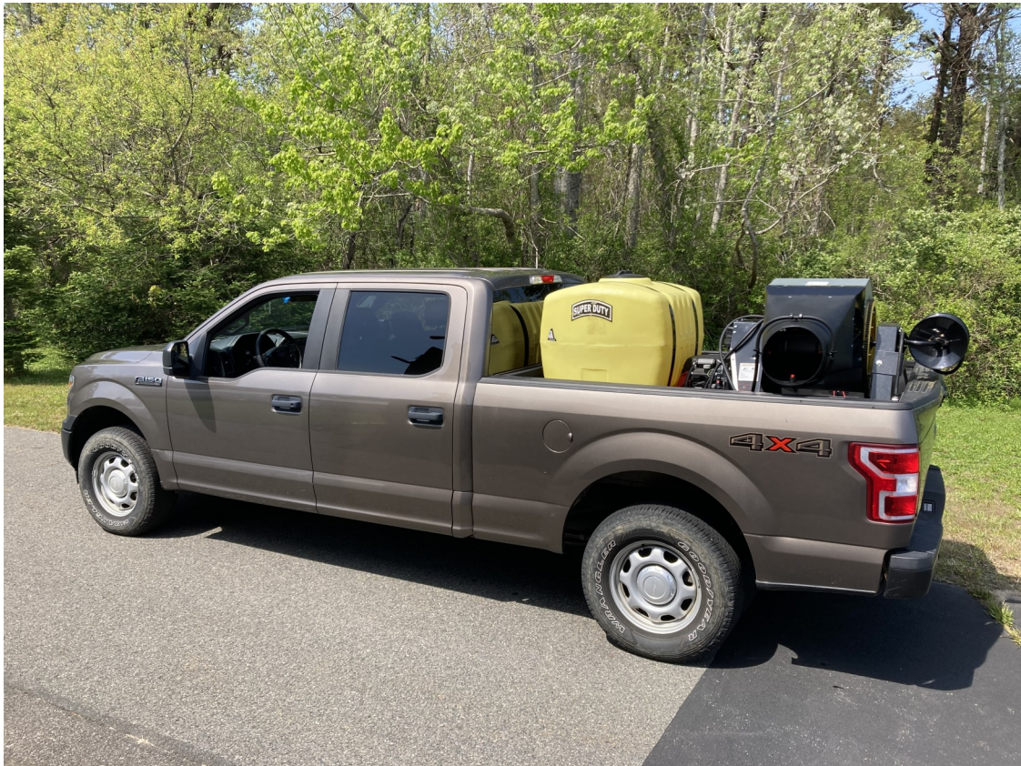
Figure 1. A1 “Super Duty” mist sprayer set up on a vehicle for field use.
