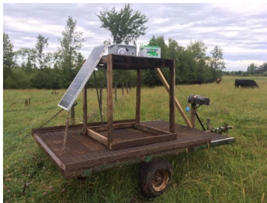
Figure 7. Mobile scare radio electronic deterrent device for wolf damage management.
