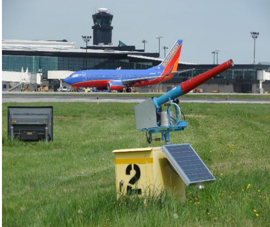
Figure 6. Propane cannon installed on an airport greenbelt to deter birds.
