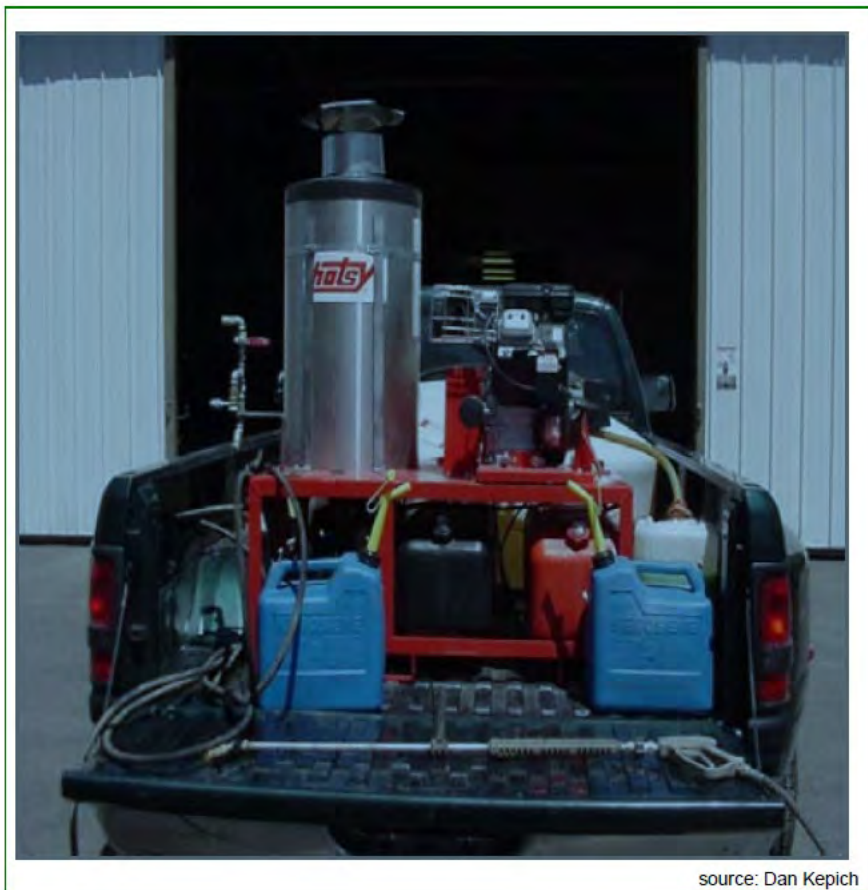
Figure 7-3 Pressure-Washing Equipment and Supplies
